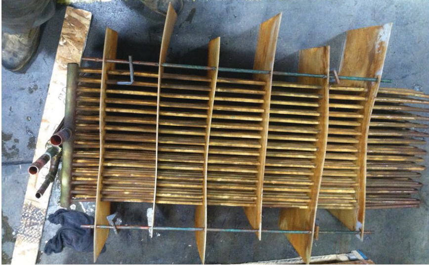
This evaporator coil corroded because glycol and inhibitor were not used during operation, which resulted in calcium buildup.
